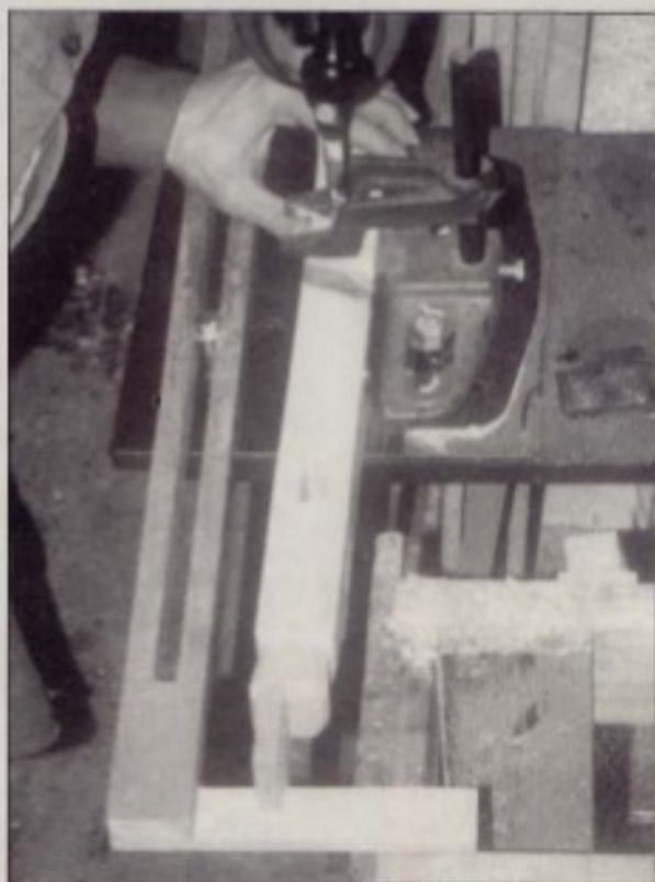
Chavez uses this stop to locate the mortises. A spacer that hangs from the stop sets the second position of each mortise.
