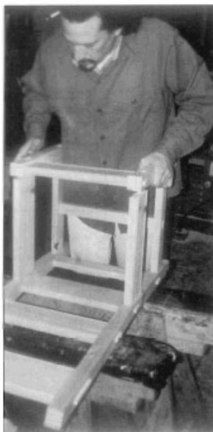
Make the front and back subassemblies; then add the side rails and stretchers.
